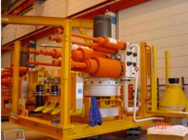
XMT 1 in FAT (small bore removed)
