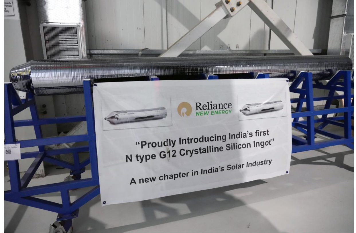
First Ingot (300 mm diameter and 2.85 m length)
