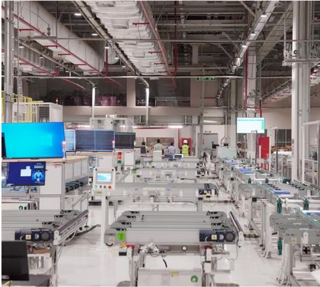
Pre-lamination Testing Station [including Electroluminescence (EL)]
