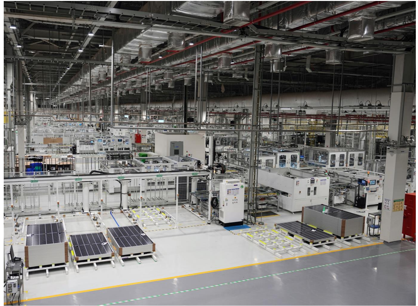
Post-lamination Area [including Junction Box application, framing, testing, sorting, etc.]
